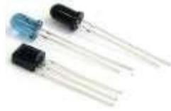
Gambar 18. Hight Emiting Diode (Dioda Emisi Cahaya)
