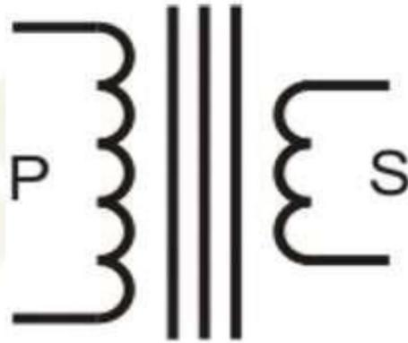
Gambar 35. Simbol Transformator Step Down
