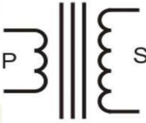
Gambar 34. Simbol Transformator Step UP
