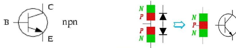
Gambar 15. Transistor NPN
