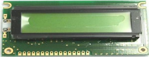
Gambar 26. *Liquid Crystal Display (LCD)*
