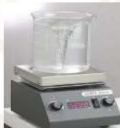
Gambar 1 *Hot Plate Magnetic Stirrer*
