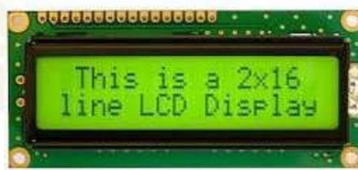
Gambar 2. 9 LCD 2x16
