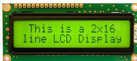
Gambar 49 LCD 16 x 2
