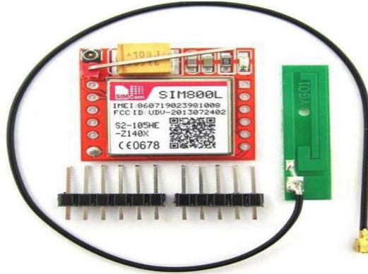
Gambar 6. MODUL GSM SIM800L
