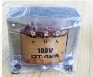
Gambar 33. Trafo Output/Input
