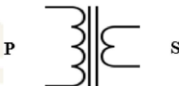
Gambar 15 Lilitan Transformator Step Down
