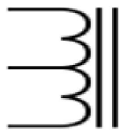
Gambar 16 Lilitan Transformator Autovariabel
