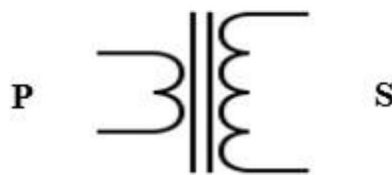
Gambar 14 Lilitan Transformator Step Up
