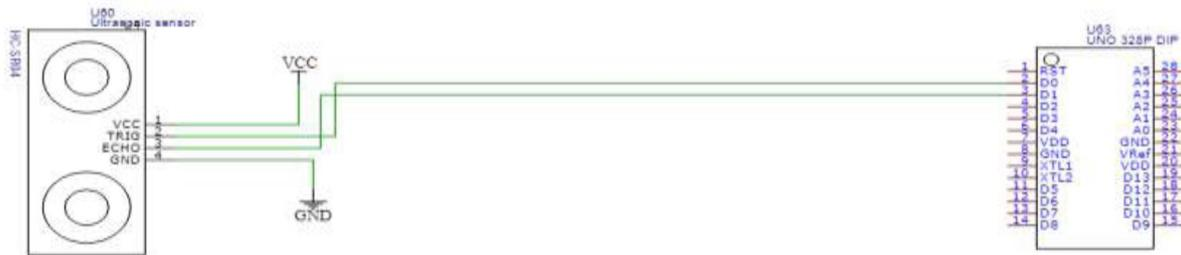
Gambar 3. 4 Rangkaian Sensor Ultrasonik HC-SR04
