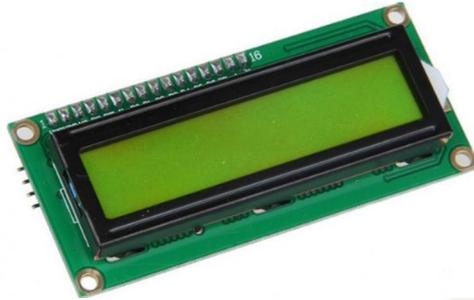
Gambar 24. Liquid Crystal Display (LCD)
