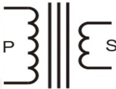
Gambar 4. Simbol Transformator Step Down
