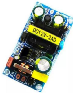
Gambar 20 Power Supply Switching
