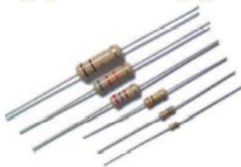
Gambar 15 Resistor Arang (Carbon Resistor)
