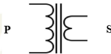
Gambar 12. Lilitan Transformator Step Down
